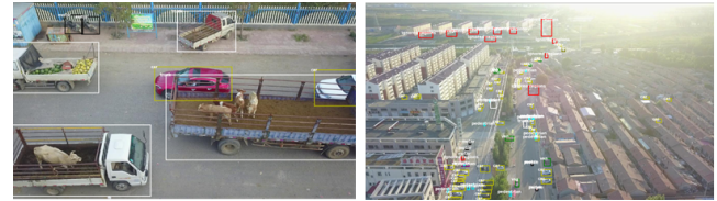
Fig. 1. Two different images demonstrating sample challenges in aerial datasets: different viewing angle and objects appearing in much smaller size. Images are taken from the VisDrone2019 [6] dataset.
